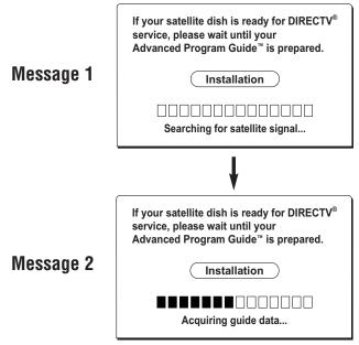
4. If Message 1 does not appear after 30 seconds, press the remote control's **SAT** button. Then press the remote's **PWR** button. The receiver beeps twice and its Antenna Power light comes on.
